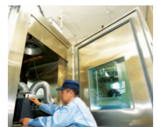
HALT Highly accelerated life test (HALT): Test to confirm the thermal and vibration limits.
